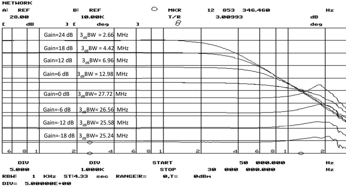
**PGA2, All gain settings, Load= 1M Ω VDD=3.3V**
