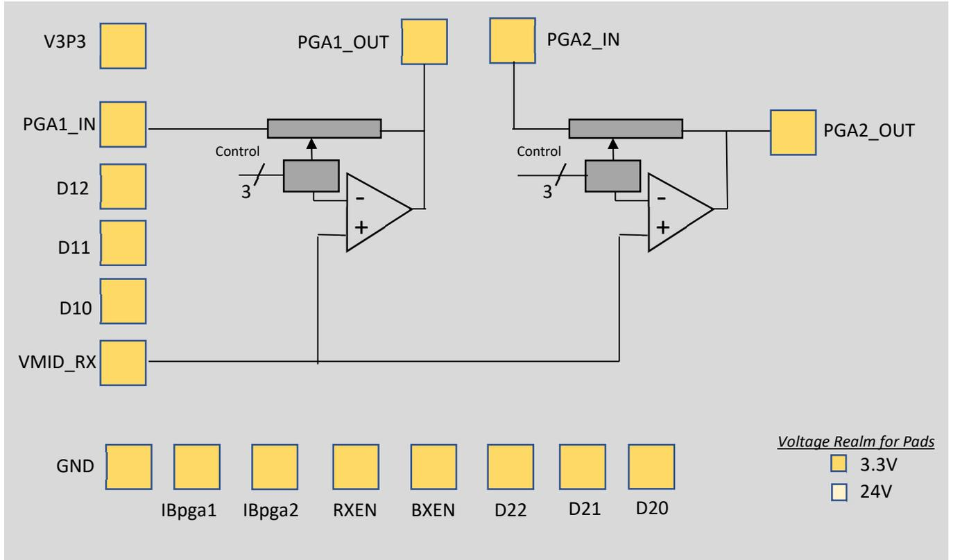
Three bits are used to program the PGA1 to gain settings from -18 dB to +24 dB in 6 dB steps. There is a power down state that allows PGA1 to be powered down when not in use allowing a low-power state for TX or RX.
